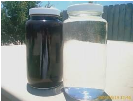
Pit water before (left) & after (right) Bear Creek Services' process of FO water reclamation.
